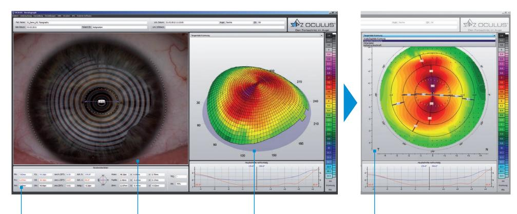
Keratometric data, diameter of the cornea and pupil, K-values and index for keratokonus detection, size of the analysed surface Built-in measuring instrument for measurements in the camera image
