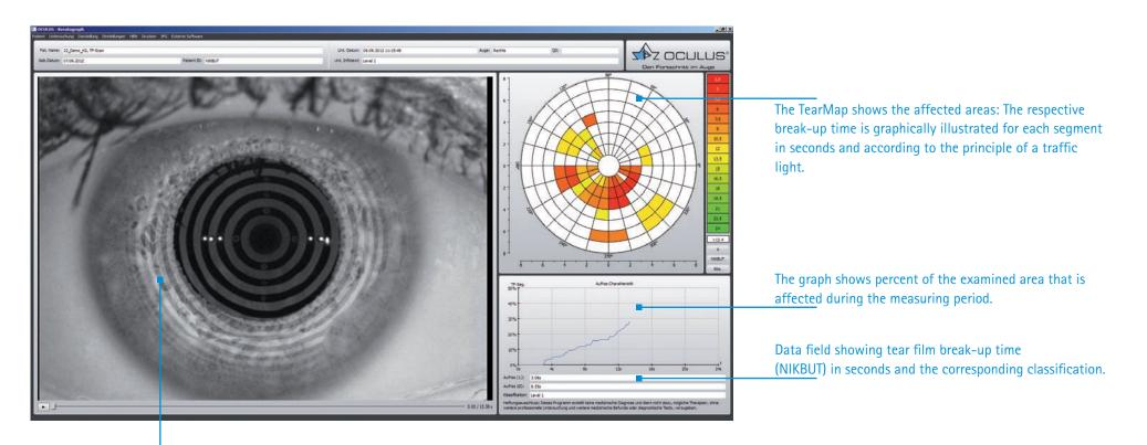
You can watch the video after the measurement. The break-up areas detected by the software are highlighted accordingly.
