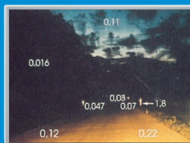
> Luminance values of street scene at night in \text{cd/m}^2
